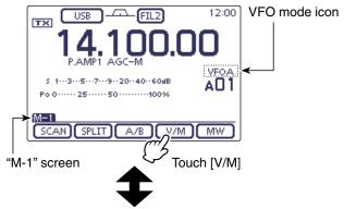
Programming 10.12000 MHz/CW into Memory channel A01.
