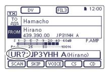
This means that your gateway call was correctly sent from the "Hirano" repeater to the "Hamacho" repeater.
